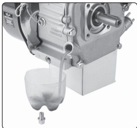
Fig. 9. illustrative picture of positioning of the engine for draining oil
